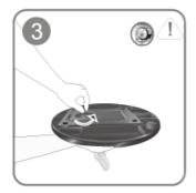
Turn the connecting screw at the bottom of the stand to separate it.
